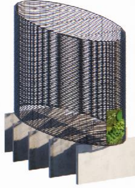
DETALLE 3 - COLOCACION DE JARDIN VERTICAL WIFFERUSSE D.50X1.00X
