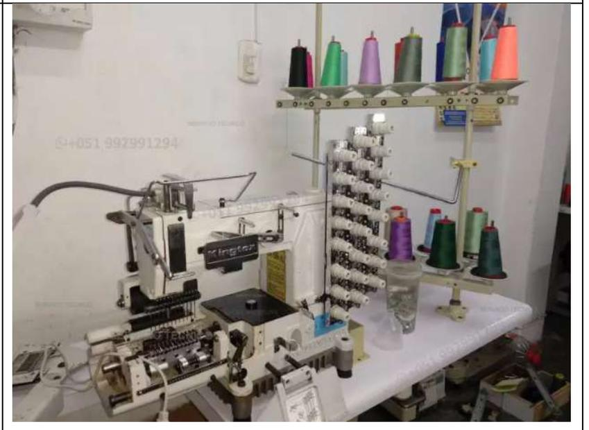
A multi-needle sewing machine is shown on a white table. The machine has multiple needles and is designed for creating decorative stitches. A rack of spools of thread in various colors (red, green, purple, blue, orange) is mounted on the wall behind the machine. A phone number "+051 992991294" is visible on the wall. The machine is a complex piece of equipment with many adjustable parts. |
