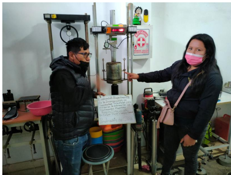
Figura 23. Prensa del Californian Bearing Ratio
