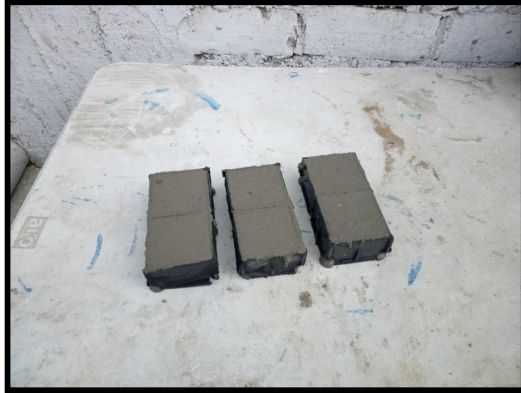
Figura 42. Vaceado de concreto (Laboratorio quality control express s.a.c)
