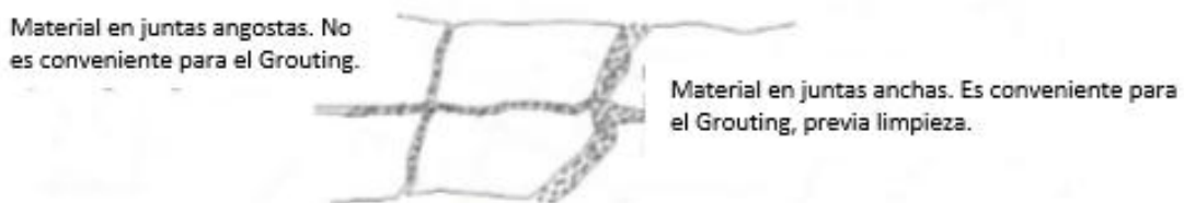
Figura 14. Tendencia al Grouting.
