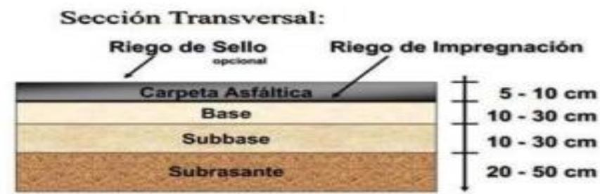
Fuente: (AASHTO, 1993 "Guide for Design of Pavement Structures 1993")
