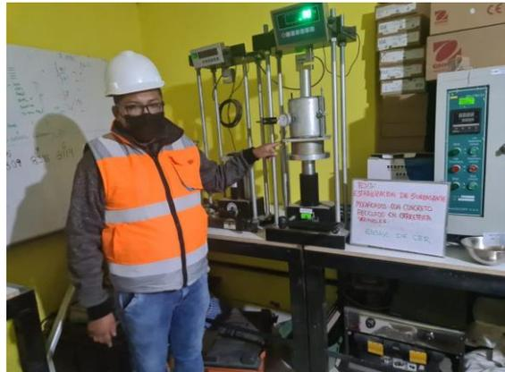
Figura 36. Ensayo de Californian bearing ratio
