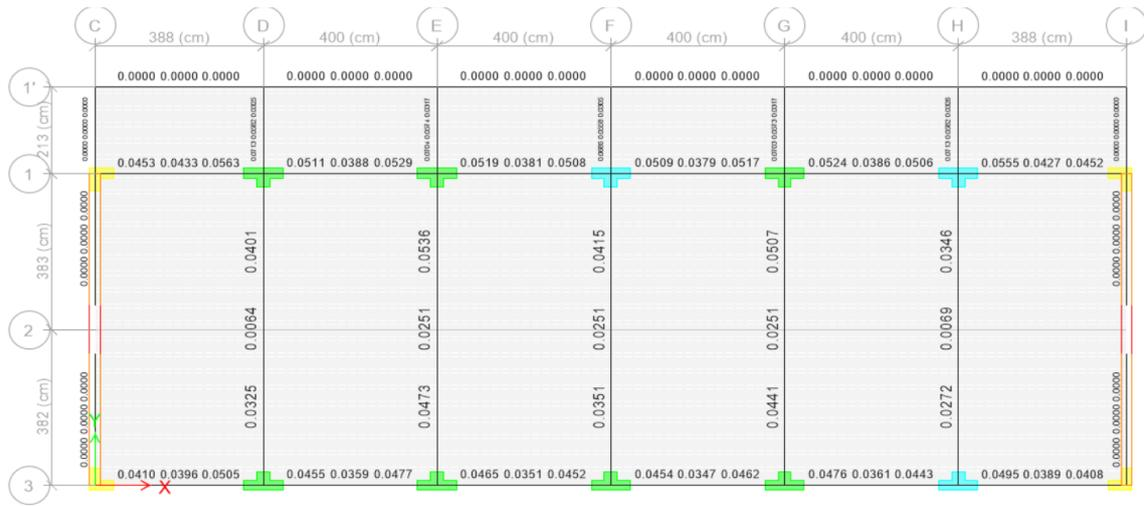
**Figura 129.** Acero Requerido Transversal (cm<sup>2</sup>)
