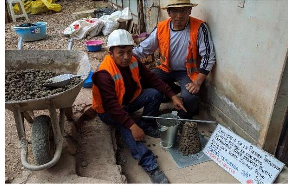
Slump del concreto permeable
