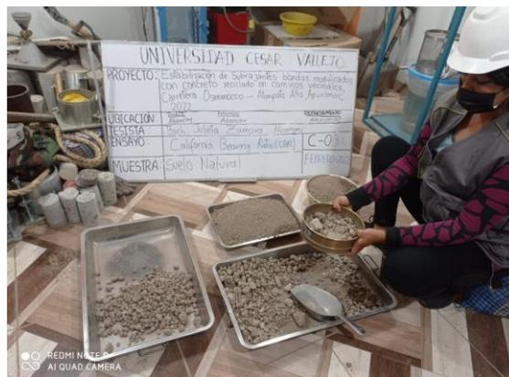
**Figura 3.14.** Ensayo CBR, SN, C3
