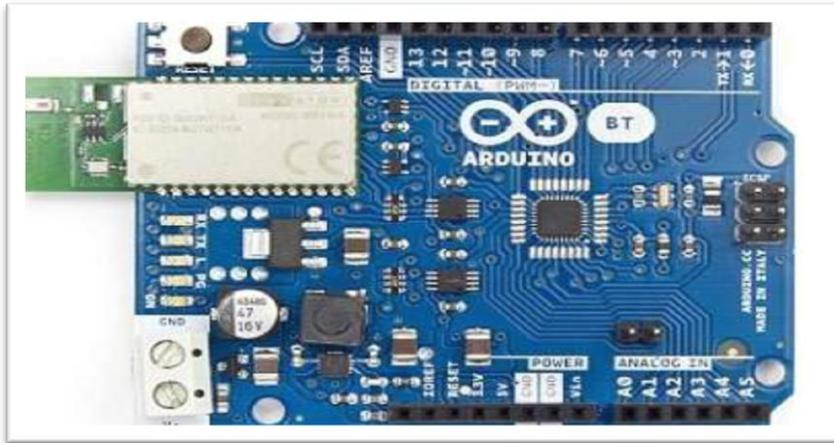
Figura 13: Arduino Bluetooth (Robotics, 2012)
