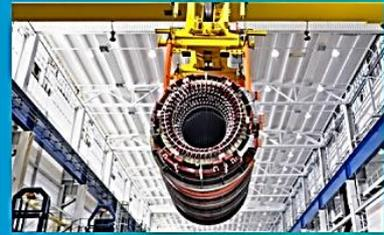
Siemens is using Global Vacuum Pressure Impregnation (GVPI) technology for manufacturing robust and maintenance free generator stators
