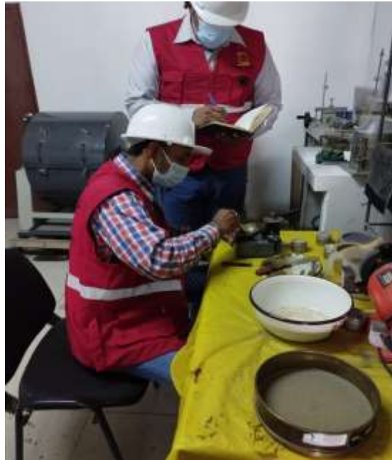
Figura 29: Agregando material a la cuchara
